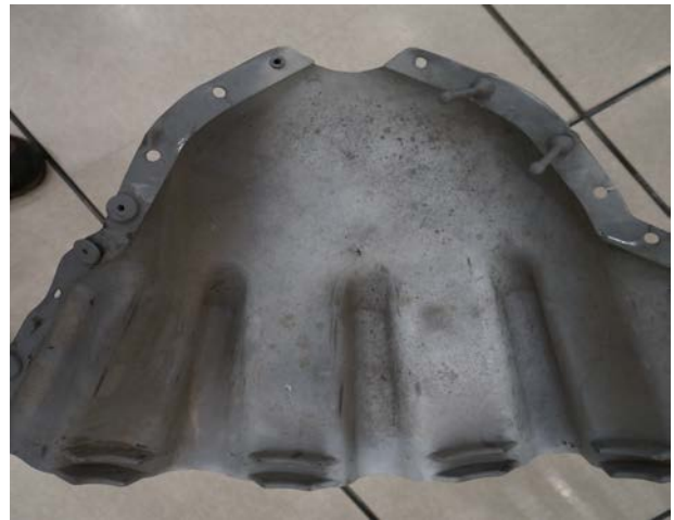
Contamination on inside of E/Bushing cover.
